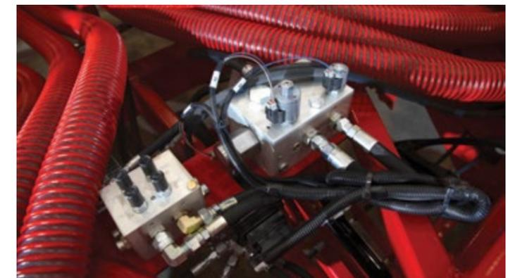
This new hydraulic system is compatible with the Topcon X35 control system which adds Autolift, a feature that automatically lifts and lowers openers at headlands and Autopack, a system that allows the user to change opener packing force on the X35 monitor.
