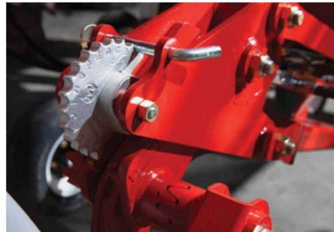
The Quantum row unit features a depth shim system to allow for deeper seeding. There is a removable shim under the depth cam and removing the shim results in an increase in 1 inch seeding depth.
