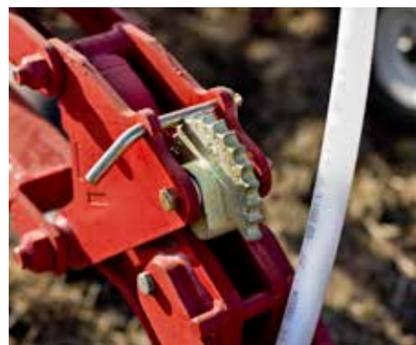
The C2 Contour opener cam is higher and away from the ground so opener adjustments are much easier to make. The notched cam-and-pin system is at 1/4 inch intervals. Rotate the cam by hand and insert the pin to lock in the desired seeding depth.
