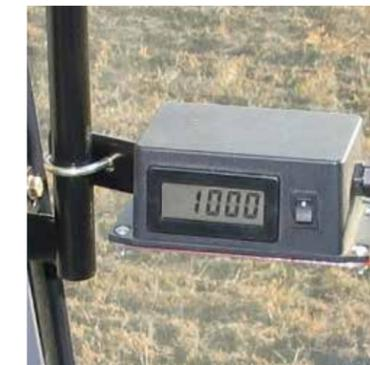
Once set, pressure can be adjusted from the tractor cab on a convenient digital display.
