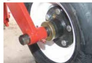
An enclosed shield and seal protects the hub bearings from mud and debris.
