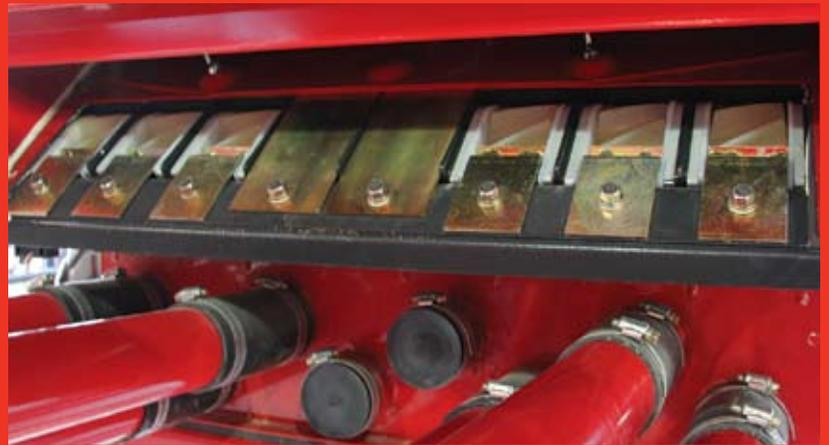
From the Air Cart to the ground, Morris provides advantages that are unmatched by competitors. Unique spiral fluted metering wheels gently roll product into the air stream in a constant flow - providing a distinct contrast to the uneven dumping of straight fluted metering wheels.
