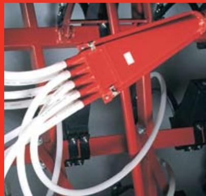
The smooth horizontal flow of material is retained by Morris' patented Flat Fan Divider Head, which eliminates abrupt direction changes found in vertical divider heads. The Morris system minimizes seed damage, reducing input costs and increasing yields.
