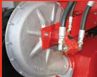
On the MORRIS system, product does not have to be lifted and experiences no 90-degree bends or sharp turns, so only one fan is required to move product from the meter bodies to the ground. An industrial piston-type hydraulic motor powers a 13" (33 cm) diameter forward curved fan that is 98% efficient. Use of larger hydraulic lines decrease flow restrictions for less heat buildup under higher fan speeds.
