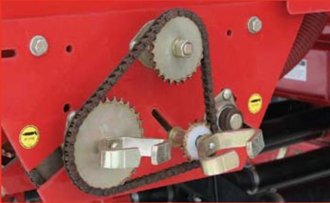
Posi-Drive Transmission - using a positive lock on all drive sprockets to deliver smooth and reliable metering. The positive ground drive from the air cart wheel compensates for any changes in ground speed, ensuring precise product rates at all times.
