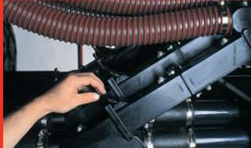
Morris' innovative design makes it convenient to switch between single and double shoot with a flip of a lever. The Diverter Valve allows the product in each tank to combine evenly into one air stream. Or, you can choose to keep the product separate.
