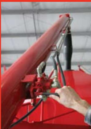
The 7000 Series auger is double-hinged for exceptional balance, allowing one person to easily load and unload. The 7180 model is equipped with a 7" auger. The 7240 and 7300 models come with 8" auger.
