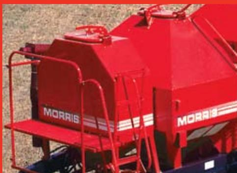
The Granular Tank option allows you to broadcast granular herbicide on the soil surface, while accurately placing seed and fertilizer at two different levels in the soil.
