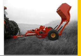
Highline is the only rock picker with the box frame construction. The front frame is built high to let rocks in yet ensure the structure is strong enough to withstand the most difficult rocks that are removed from the field.
