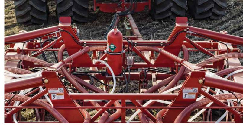
Pressure is maintained on the opener cylinders through a passive hydraulic system that uses a hydraulic accumulator. This unique hydraulic accumulator system acts as a hydraulic cushion for the trips, and being a passive system, greatly reduces the demand on the tractor hydraulics compared to the continuous flow required by similar drills. By adding or subtracting oil from the accumulator circuit, through a tractor
