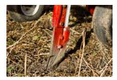
The true one-to-one parallel linkage maintains a constant opener angle relative to the soil and constant opener depth relative to the packer wheel throughout its 17-inch range of travel. The opener can contour up 10 inches and down 7 inches.
