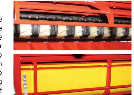
system. The spiral flute provides a continuous flow of product into the air stream. All-in-one seed plates save time, one quick change lets you accurately meter fine, medium or coarse products.
