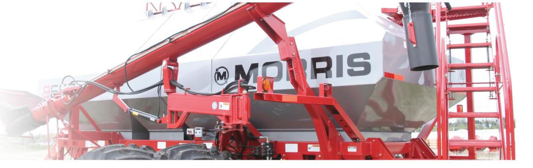
Achieving the perfect balance of reliability and precision, the new 9-Series Air Cart comes with a list of next generation innovations. Advancements include Input Control Technology, new tank configurations, a left-side auger for easier access, a redesigned stairway and the Topcon X30 console.
