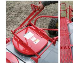
The improved lid design incorporates a gas cylinder to assist the operator when opening and closing the tanks. The handle is also repositioned so the operator does not need to stand above the lids to open them. The lids can then rotate to sit along the tank panel and reduce clutter on the walkway.
