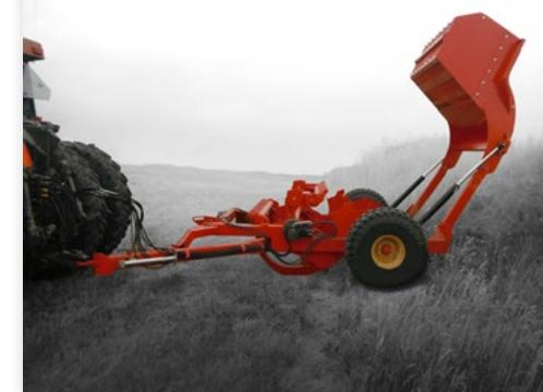
Highline is the only rock picker with the box frame construction. The front frame is built high to let rocks in yet ensure the structure is strong enough to withstand the most difficult rocks that are removed from the field.
