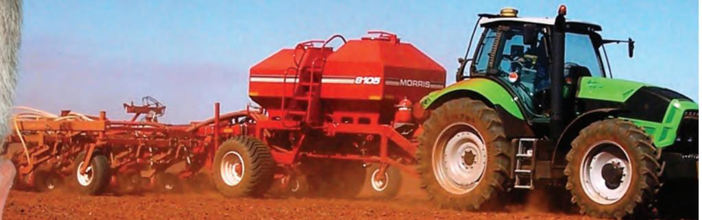
The CX 8105 seeding system combines the precision of the Contour independent drill with the seed metering accuracy and efficiency of the Morris air cart.
